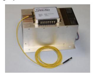
The integrated cooling system (ICS) if purchased without the SemiNex multi-chip module (MCM) is shipped as a stand alone entity with pre-tapped holes to accommodate the MCM. The ICS is comprised of a heatsink and convective cooling fan fully assembled. The dimensioned drawing appears in figure 1.
